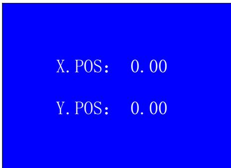
Press to delete the “X. POS” value and enter the new value with digit keys; press or to move the cursor to “Y. POS”, press to delete the “X. POS” value and enter the new value with digit keys. Press to save, press again to confirm.
